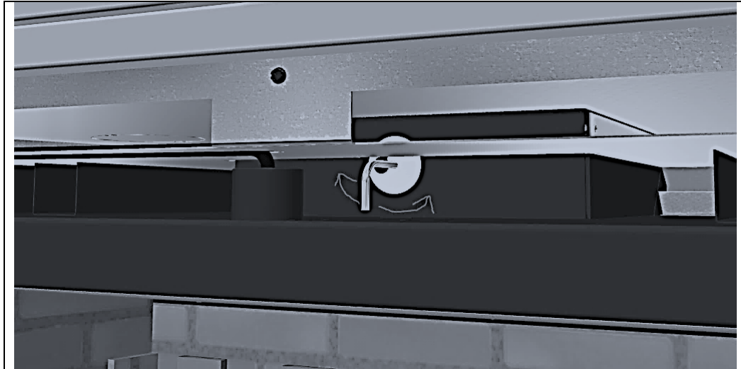
Figure 4-21 Exhaust Damper Adjustment
